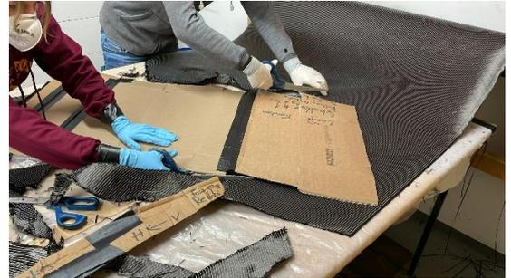
**Chassis** - We have made great progress in the last two months: We have now finished the first half of the carbon negative mould of our monocoque. In addition, the laminate structure has also been completed. In the next few weeks, the second half of our mould will also be manufactured and various material tests of the laminate structure will be carried out.
