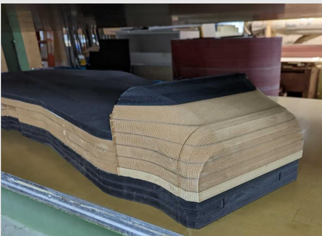
Our positive wood mold during milling.
